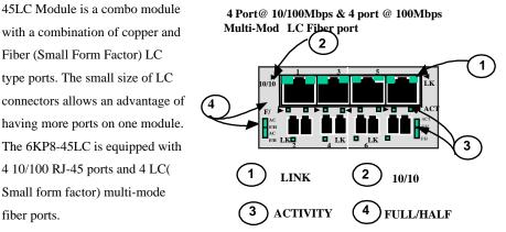
When installed in a Magnum 6K32T Switch, it supports the standard distances as per mentioned on 5.2.8. and the LEDs also acts similarly as mentioned above.
